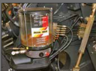
Automatic greasing system
