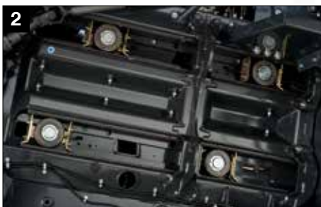
26 Heavy duty - greased plunger rollers
