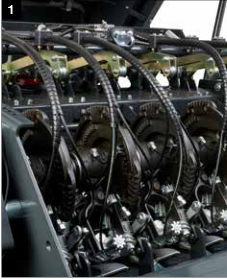
1 Double knotting system with standard electronic monitoring
