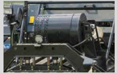
Hydraulic driven turbo fan (only for LSB 1270)
