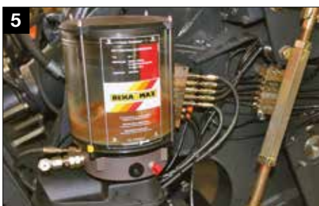
Automatic greasing system
