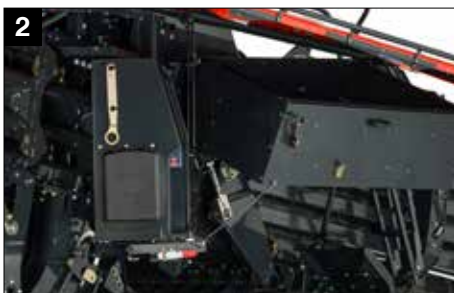
2 Pivoting twine boxes for easy maintenance
