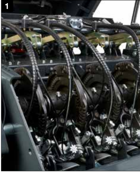
Double knotting system with standard electronic monitoring
