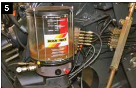
5 Automatic greasing system
