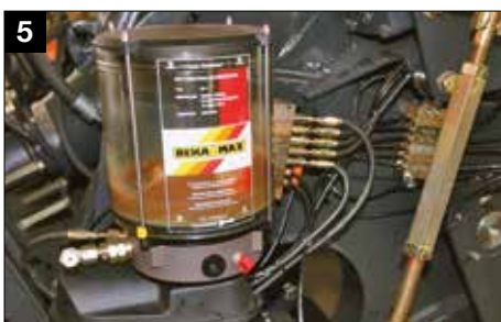
Automatic greasing system
