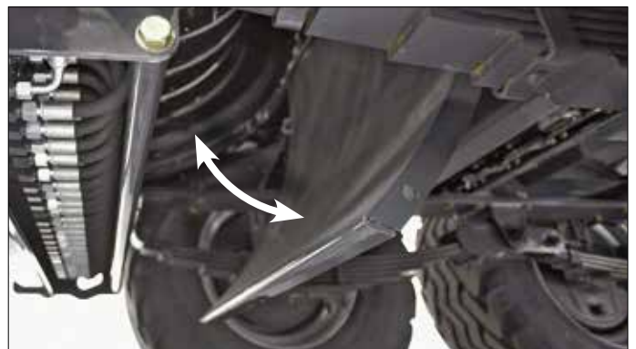
Pre-chamber inspection door
