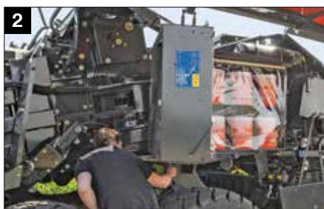
Pivoting twine boxes for easy maintenance
